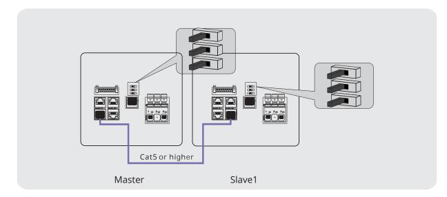
The connection diagram of two battery systems could be read below.
