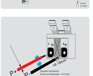
Cross Section Area: 6-16 mm<sup>2</sup> For the right cable cross section, please check the inverter manual as well.
