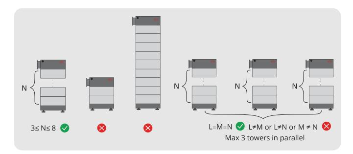
Three to eight HVL battery modules could be stacked in one tower. Maximum three battery systems could be connected in parallel.
