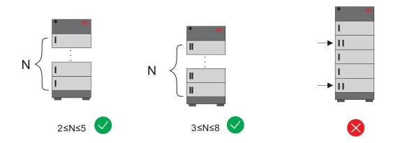
Up to maximum three battery systems could be connected in parallel. (This restriction does not apply for parallel connection with SMA Sunny Boy Storage 3.7-6.0. Please check the inverter operation manual on how to connect up to three batteries.)
