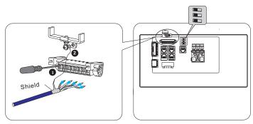
4. If necessary, trim unused insulated conductors flush with the cable sheath or fold it over the cable sheath.
